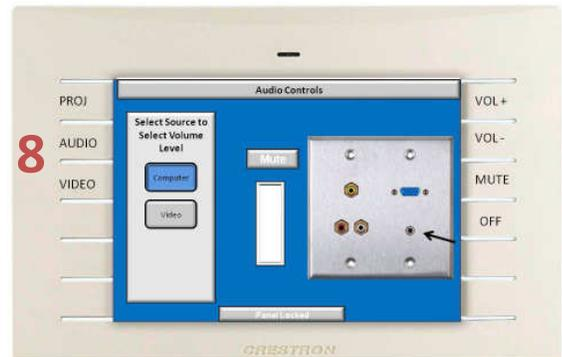
Press the touch screen button for your desired source. The image on the right will change as you select different sources.
